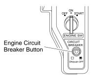
Figure 4 - Engine Circuit Breaker
